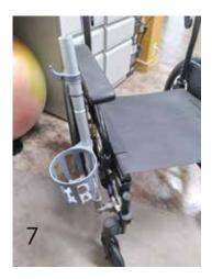
Step 7: Place the other rubber ring on the tube where you want to place the hook.
