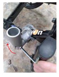
Step 3 & 4: Using the 2 smallest Allen keys position the end of the clamp into which the upright aluminum tubes will fit. Step 3 adjusts up and Step 4 adjusts left or right.
